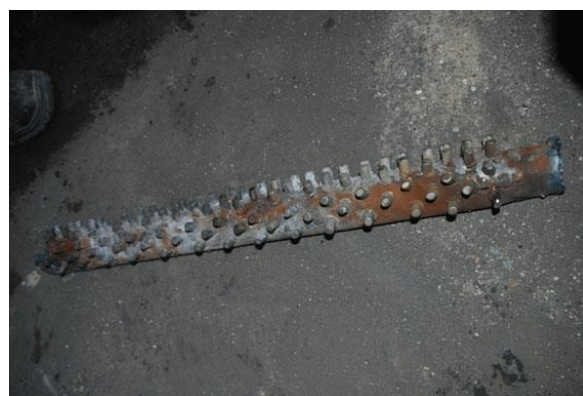
Photo 1: Failed Bed coil tube; Material Size & Specification: Ø 51 x 6.35 mm and SA 210 Gr. A1
